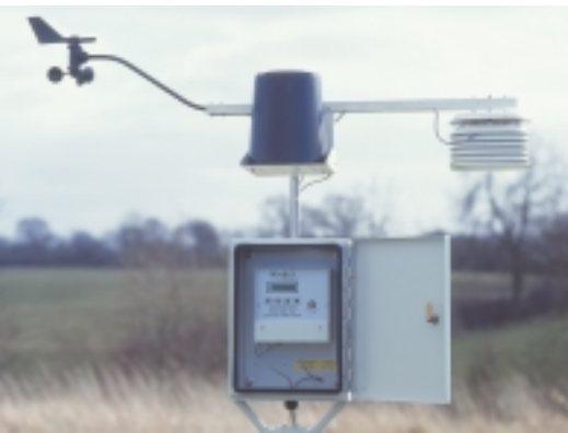
The Nimbus weather station can combine weather aspects of wind, temperature, humidity and rain fall, with the option of integrating the system into a dust monitor network. Alarm attraction systems such as beacons or sirens can be deployed.
