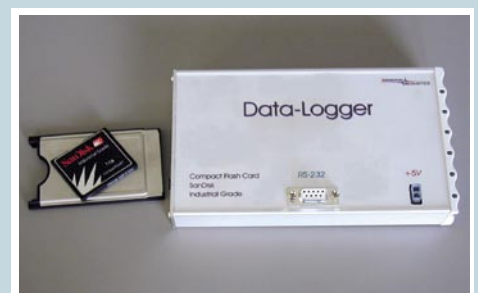
Below: Data transmission to PCMCIA-Data Logger or via Radio Module
