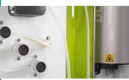
Sample water is mixed with the algae test olution and then analysed
